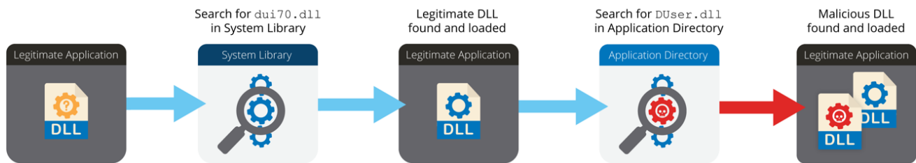
Figure 5. Chained DLL side-loading
