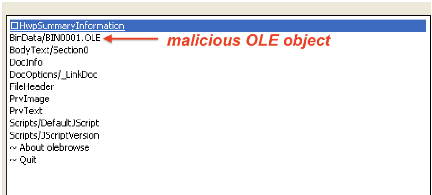
Figure 17: malicious OLE object stream present inside the HWP file
