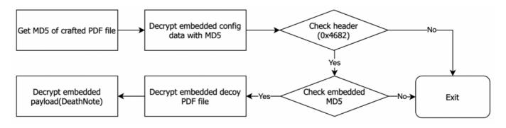
Verification process of Trojanized PDF reader
