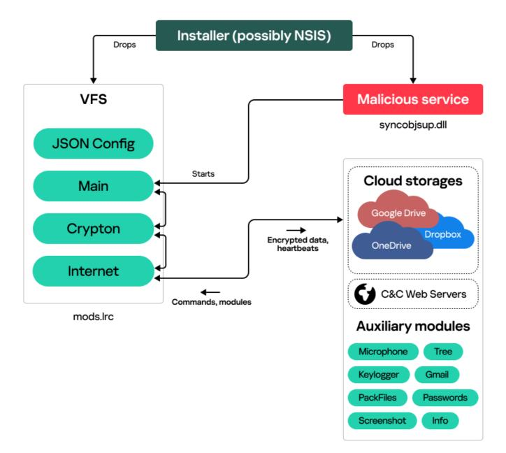
Upon launching, the orchestrator spawns a suspended WmiPrvSE.exe process and injects itself into it. From the WmiPrvSE.exe process, it makes a backup of the VFS file, copying mods.lrc to mods.lrs. It then parses mods.lrs to obtain all the framework module DLLs and their configurations. As mentioned above, configurations are JSON files with dictionary objects:
