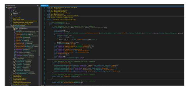
All C2 communication is encrypted using AES CBC with a hardcoded key and IV. Encryption is implemented as a separate service in the Core.Agent.Services.Implementationes namespace. Communication and command handling are implemented in a modular way using interfaces and services following common C# app development practice. To further understand the capabilities of the client we will analyze the handlers individually.
