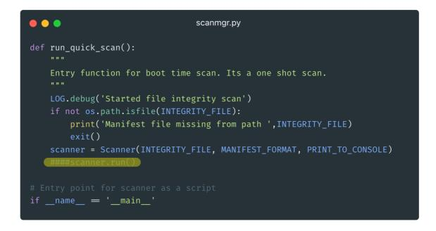
Figure 23: Scanner execution commented out in scanmgr.py
