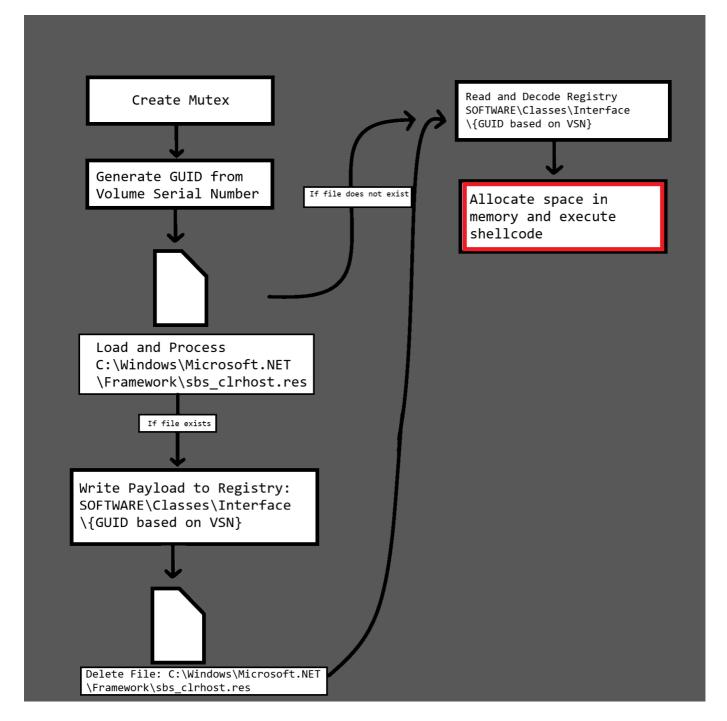
As part of the analysis, GERT identified a payload stored in the Windows registry and analyzed it, confirming the following behavior in the encrypted payload.
