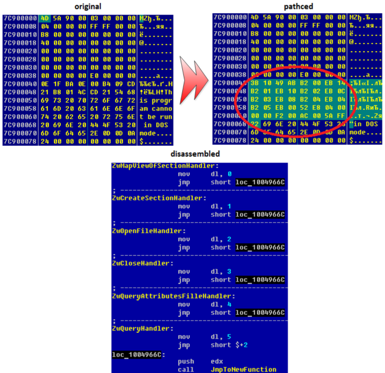
Figure 4.5 – Code Injected into MZ Header of ntdll.dll
