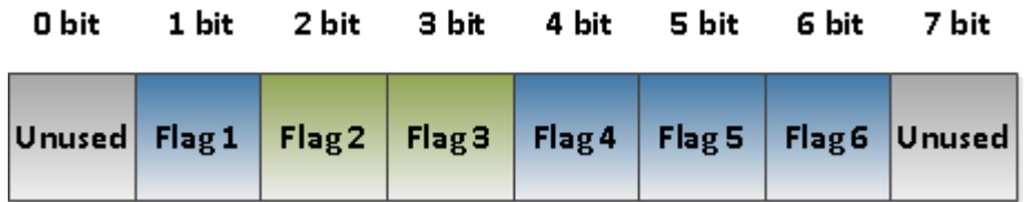
Figure 4.20 – Description of the Flags Field in STUXNET_CC_MESSAGE Structure
