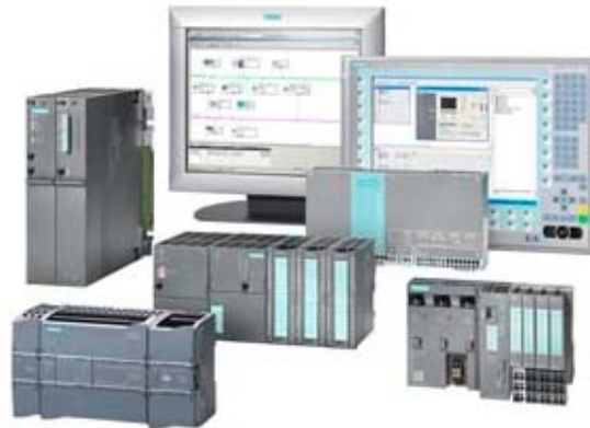
Figure 1: Some Products in the Siemens SIMATIC line, including PLCs, Operator Stations and Engineering Stations
