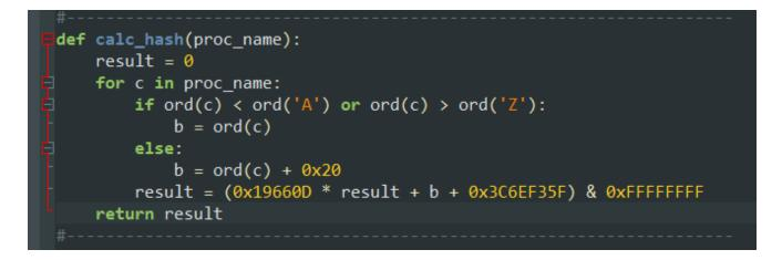
Algorithm for calculation of a hash value from a process name
