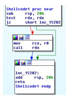
Second shellcode is a custom DLL loader, which directly loads the DLL in memory without writing it to the disk. The export is then called, with a randomly generated integer as parameter.
