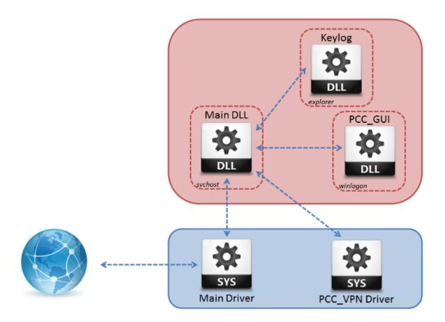
The architecture of this new Derusbi variant is distributed amongst various drivers and processes, each one being responsible of a specific task. This avoids having a single process performing all the malicious tasks, and prevents security software from raising alerts.
