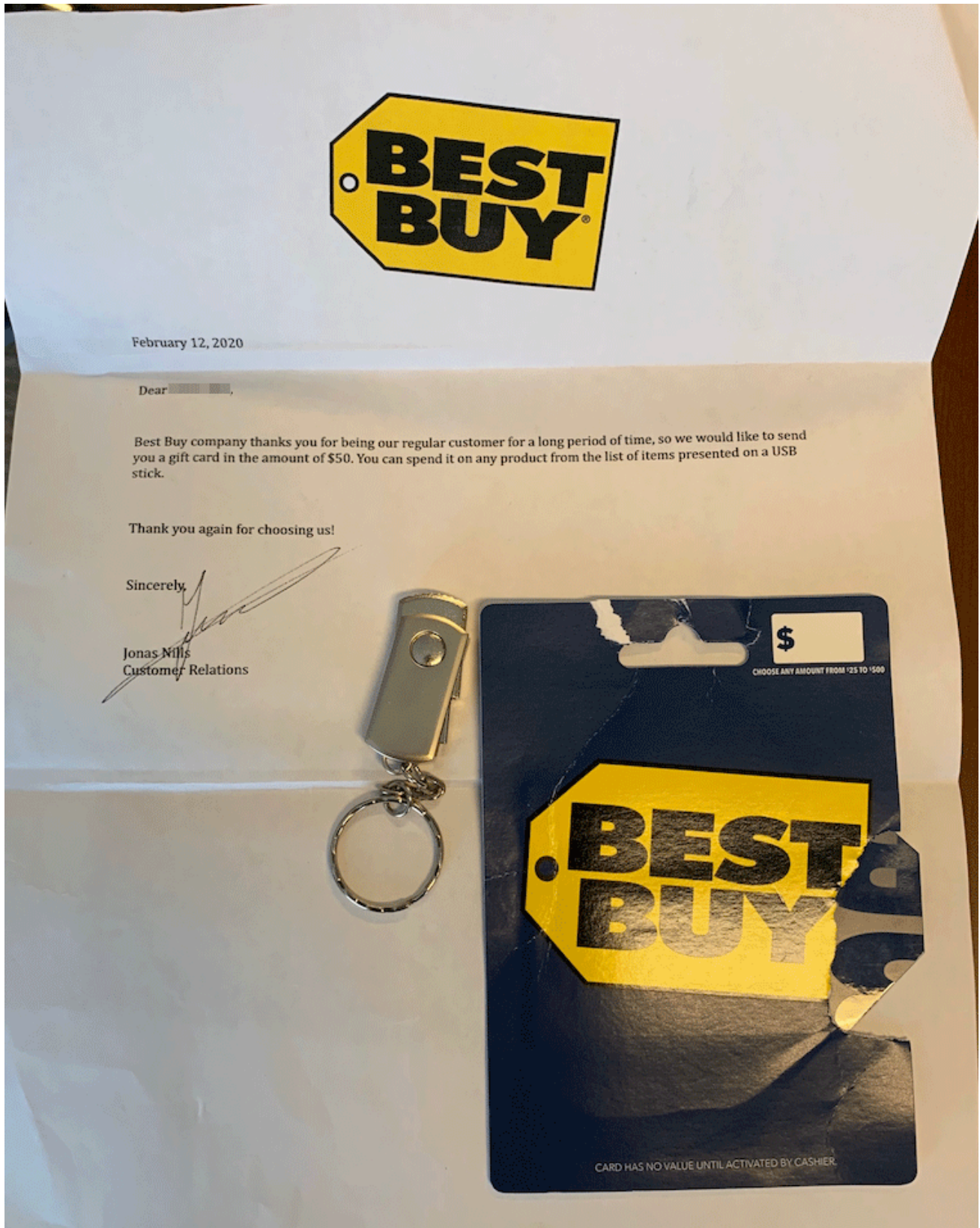
Figure 1. Suspicious Best Buy gift card containing a malicious USB device
