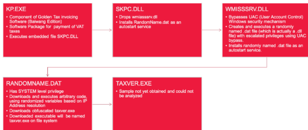
Figure 1: GoldenHelper execution process flow
