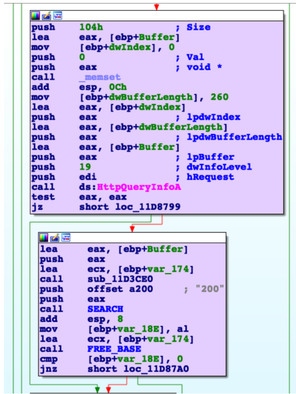
Figure 2 - Screenshot of the malware querying the C2 server after conducting the initial connection. The initial connection will pass information stolen from the target system to the C2 server, including a unique hash used as a victim system identifier. After a successful initial connection with the C2, the malware will begin attempting to download RC6 executable payloads.
