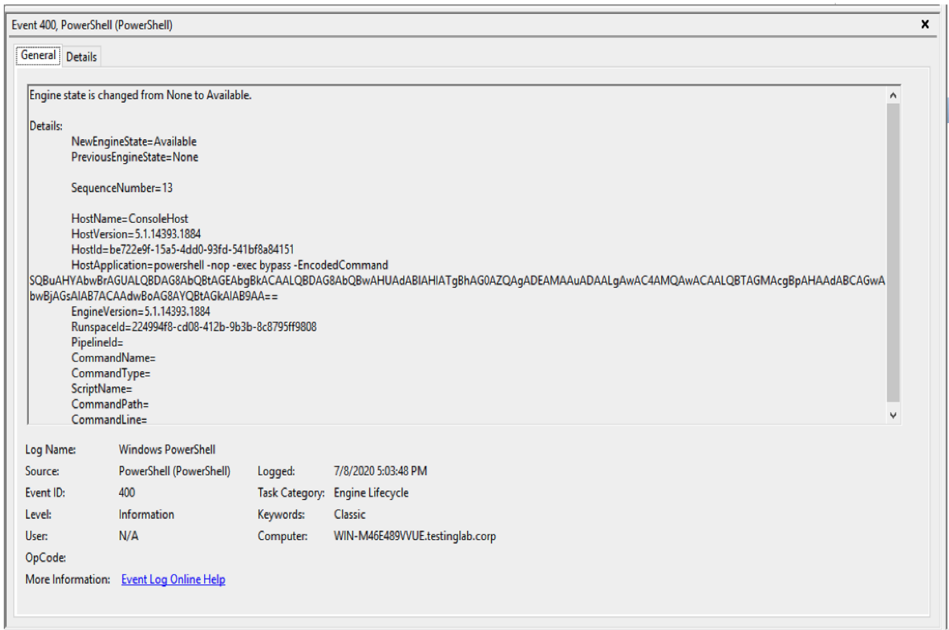
Figure 10. Artifact generated by the remote-exec powershell Beacon command when executed on the compromised system (click image to enlarge)
