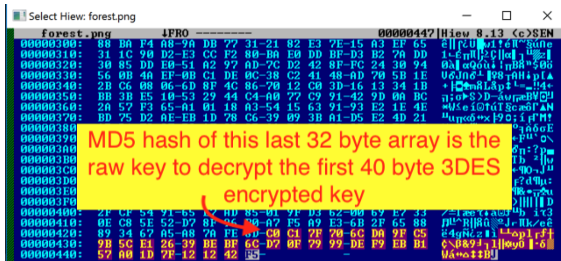
Figure 13: The last 32 bytes of the PNG file as highlighted is the KEY to decrypt the TripleDES encrypted key
