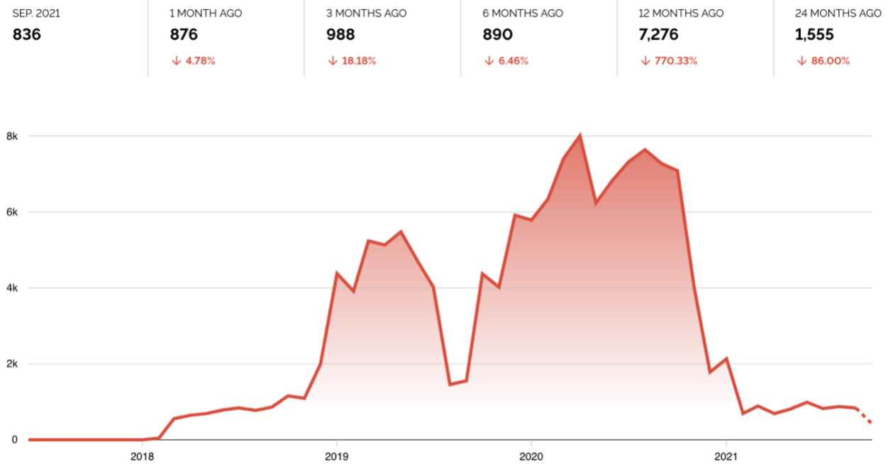
Figure 4. Shodan data showing a significant decrease in exposed Docker APIs from the latter part of 2020 to 2021
