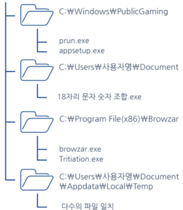
Figure 7. Similarity in file created location between malicious file in breached personal PC and malicious file distributed in topkeygen
