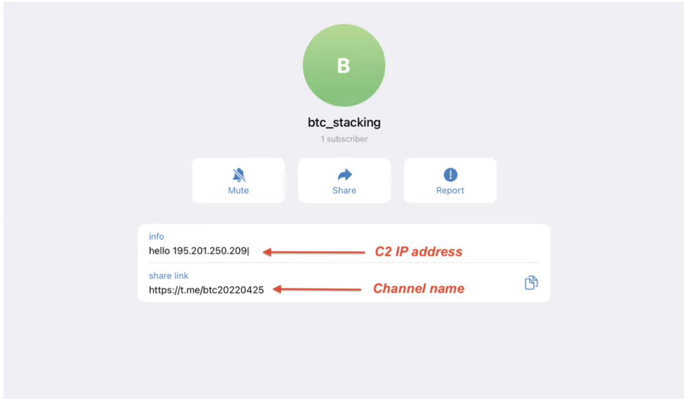
Figure 5: Vidar attacker-controlled Telegram channel with the C2 IP address included in the channel description
