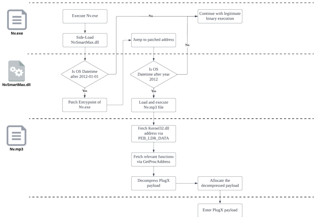
Figure 14: PlugX loader flowchart
