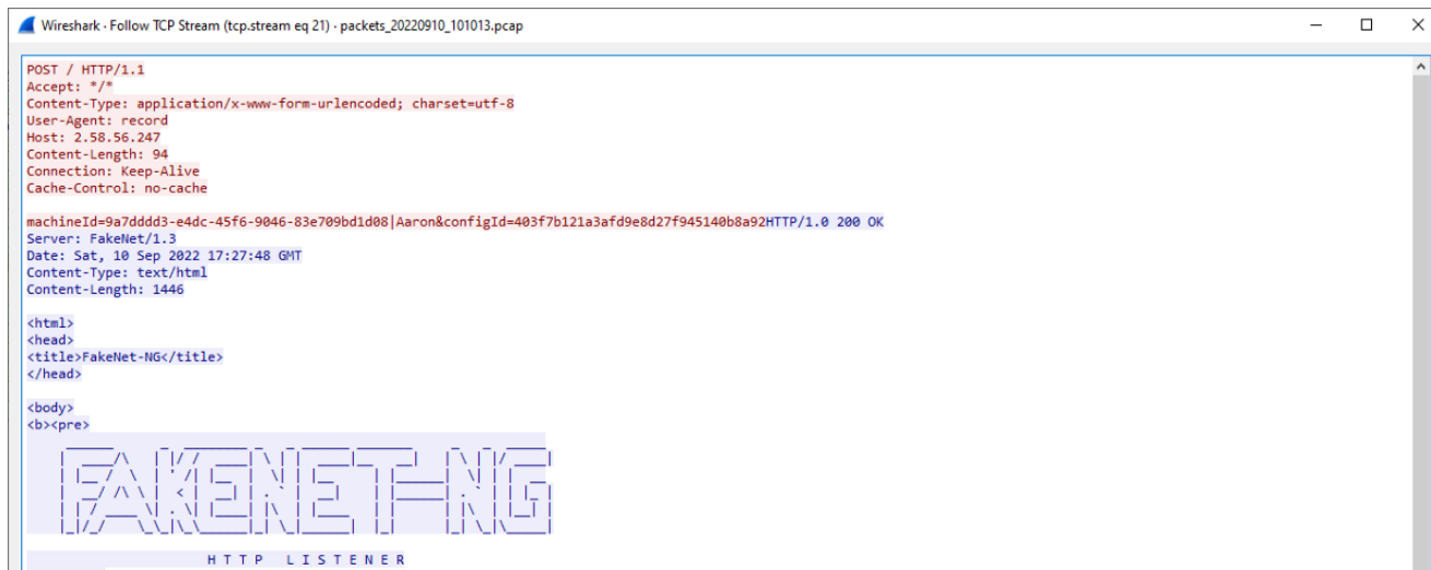
Figure 10. POST request to the C2 node containing the machineID, username, and configID parameters.
