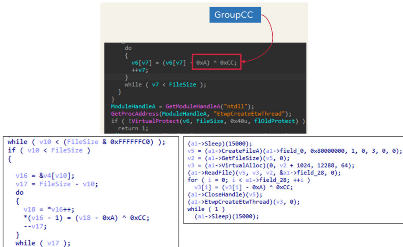
Figure 17. Decryption algorithm used by GroupCC (top), CroxLoader (left), and Symatic loader (bottom)
