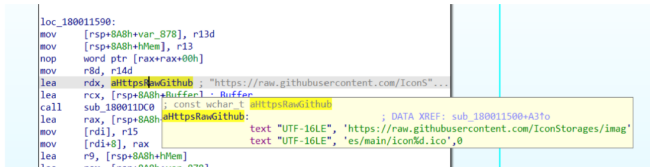
Fig.13 - Second Stage payload downloads icon files from Github Repository
