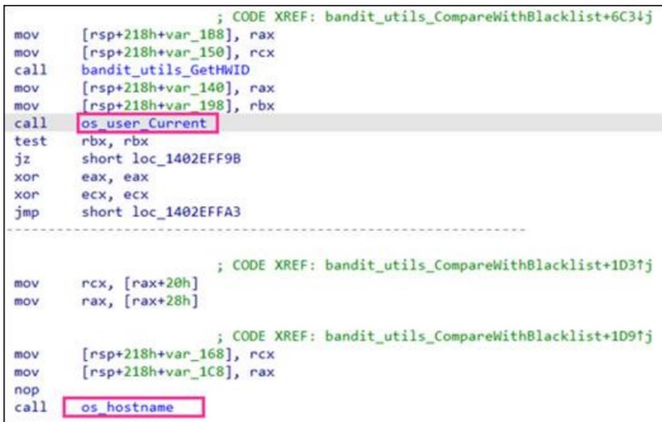
Figure 4. Bandit Stealer gets the victim's username and device name under the bandit_utils_CompareWithBlacklist function
