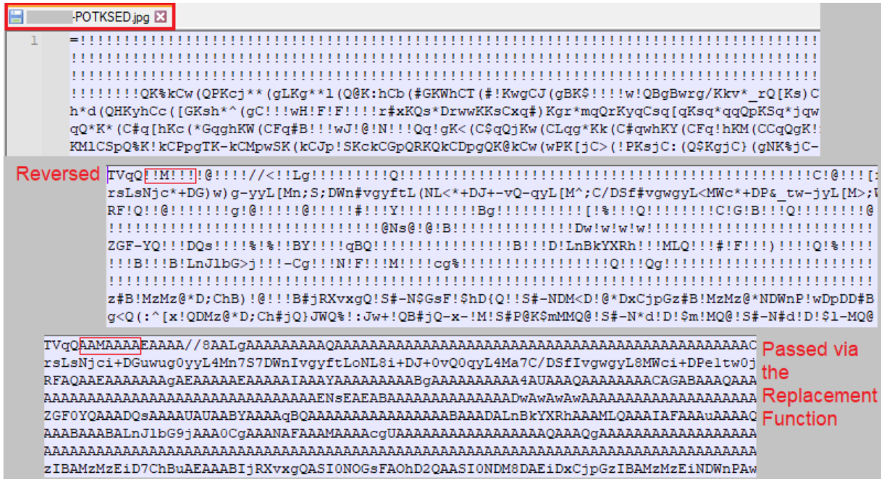
Figure 15 - Showcases the decoding process of the DLL, involving reverse and replace functions.
