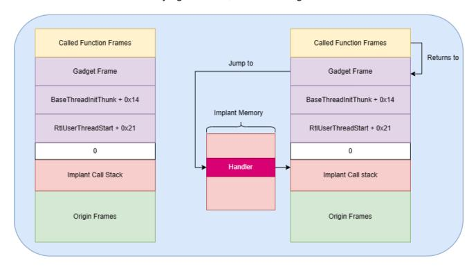
Spoofing NtAllocateVirtualMemory causes the stack to appear like below.
