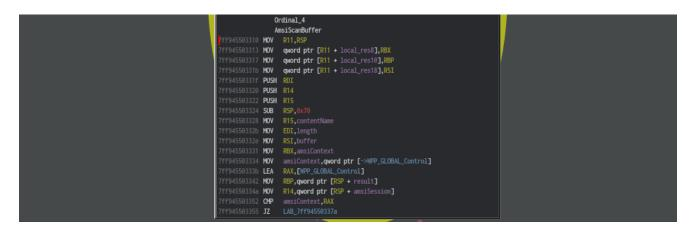
here we can see stack pointer is stored in **r11** register and since this is x64 \_stdcall, the first four parameters are stored in rcx, rdx, r8 and r9 registers. Rest are stored in the stack. With that information, we can assume a pointer to the AMSI\_RESULT enum is stored in the stack.
