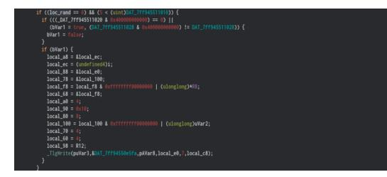
Here, the if confition only evaluate true when loc\_rand() is equal to zero and a global variable is less than 5. loc\_rand is basically the local variable where the random number was stored. Therefore this block is not going to execute.
